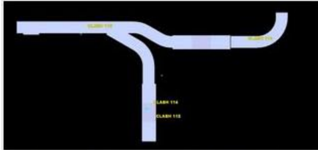
Plan view of 3d conveyor model showing clashes
