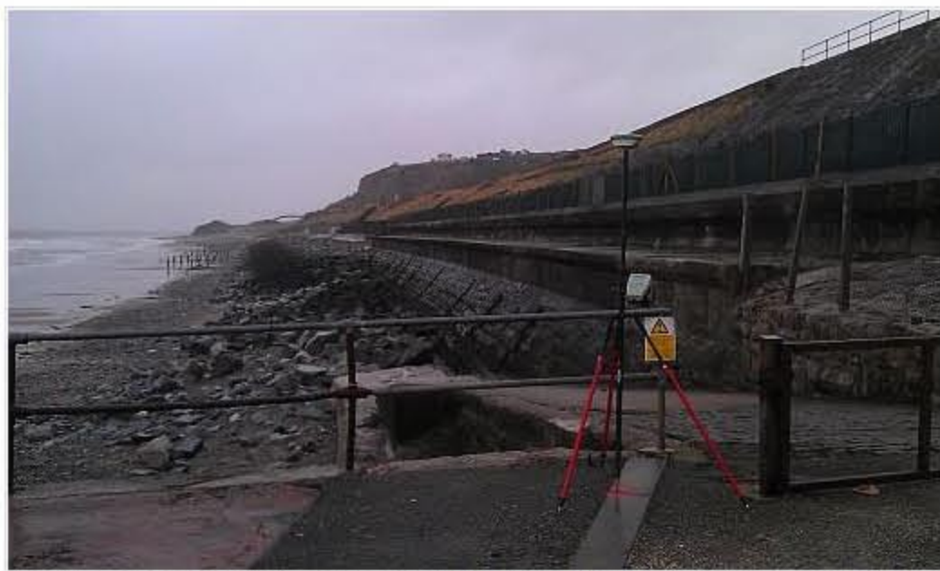
Leica Smart Rover establishing Ordnance Survey National Grid and Datum for sea wall survey
