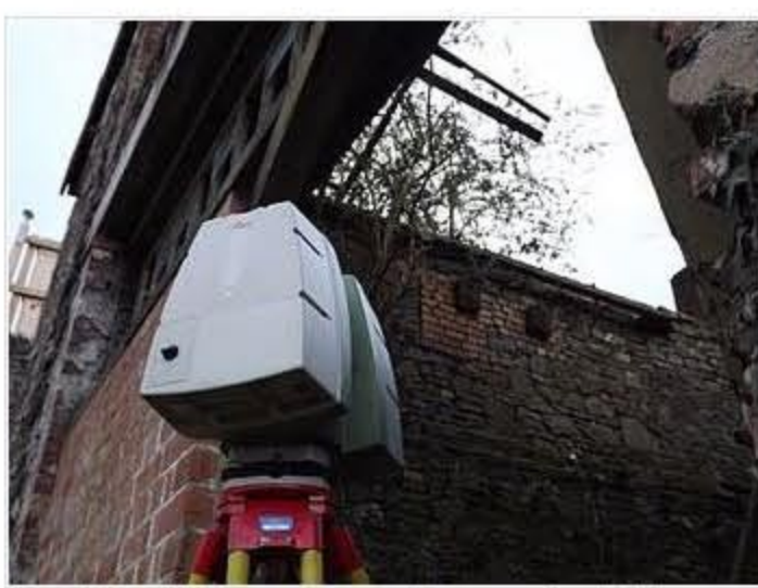
Leica C10 laser scanner used to survey the buildings
